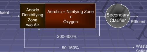
Influent → Anoxic Denitrifying Zone w/o Air → Aerobic + Nitrifying Zone + Oxygen → Secondary Clarifier (Effluent, Waste Solids)
